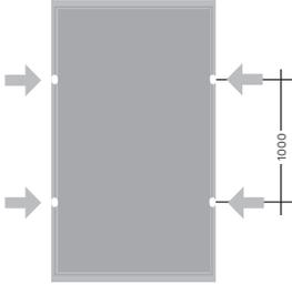
Place the clamps on the positions of the holes provided in the frame
