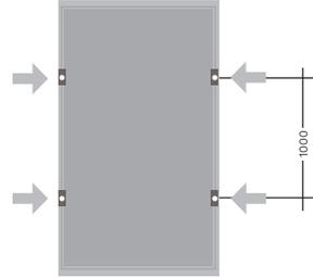
Max. permitted pressure load up to: 6,750 Pa (test load 10,125 Pa)
