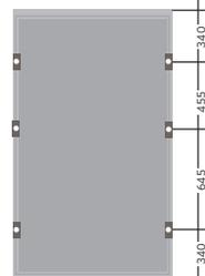
In this mounting variant, due to the high load, the module can touch the mounting rails. To avoid damage to the glass, a rubber coating must be provided on the rails.
