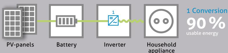
**MyReserve**, on the other hand, is installed before the inverter. It stores the direct current from the PV system. Only when the electricity is consumed in the household is it converted into alternating current. This leaves over 90 % of your own solar power available – that pays off!
