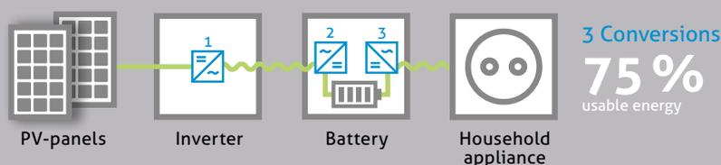
Electricity from the roof goes through an inverter and is converted into alternating current. If it is sent to a **conventional battery**, it is converted back into direct current. Then as the battery discharges the current must be converted once again to alternating current. With each conversion you lose some of your precious solar power and end up with only 75 % for your own use.
