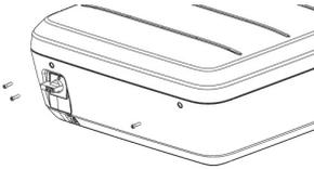
Turn the screws **(F)** into the designated holes in the base of MyReserve or its extension. One screw will need to be fastened through the switch disconnecter on MyReserve.
