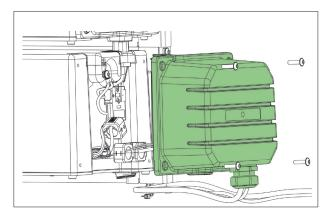
attach the protective cover to MyReserve Command with M6x22 TX30 screws (included in delivery)
