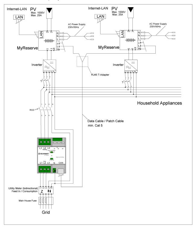
Communication coupling for the MyReserve as a cluster system is established via CAN BUS, using either Variant A (Fig.) or Variant B (Fig.).
